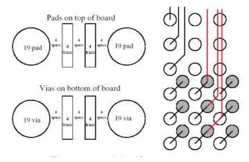
It is possible (and recommended) to divide the BGA area into four quarters. It makes the breakout escape more symmetrical and flexible.
